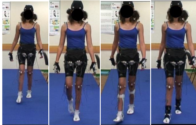
Figure 53 – Subject 2: a) IC of right foot without AFO b)MSw of right limb c) IC of right foot with rigid AFO d) IC of right foot with flexible AFO
